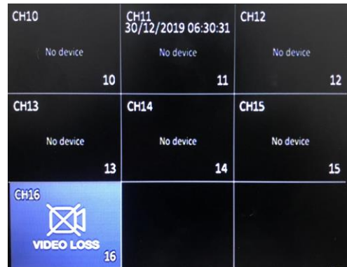
Figure 6 - IP Camera Lost Data Connection
