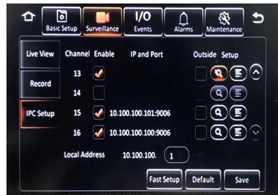
Figure 12 - IP Camera Regular Setup
