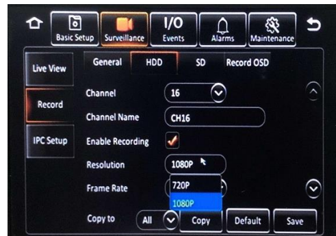
Figure 14 - Mainstream Recording Setup
